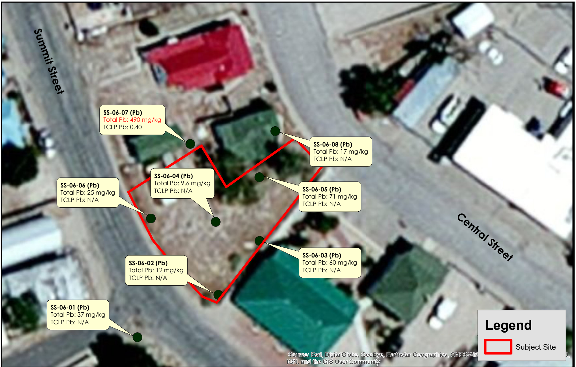
Figure 7 - Pb Soil Samples: 6 inches bgs Tonopah Library Expansion 155 Central Street Tonopah, Nevada
