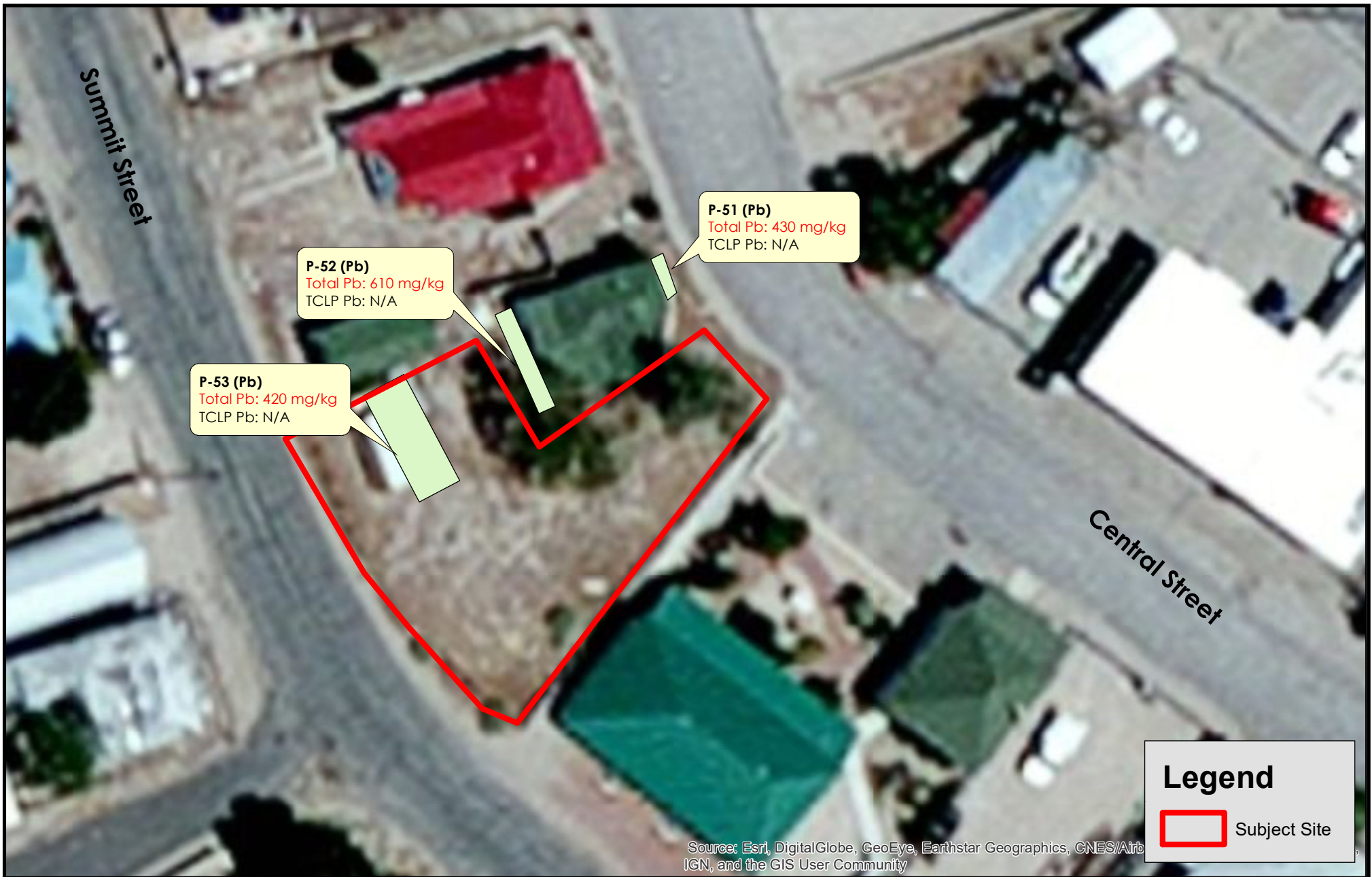
Figure 5 - Pb Soil Samples: Composite Tonopah Library Expansion 155 Central Street Tonopah, Nevada
