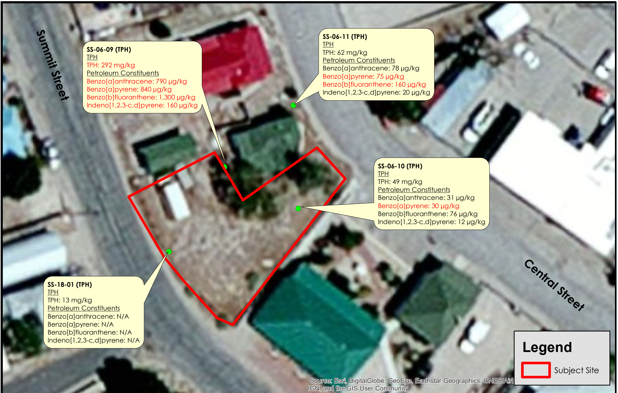
Figure 4 - TPH Soil Samples: Subsurface Tonopah Library Expansion 155 Central Street Tonopah, Nevada
