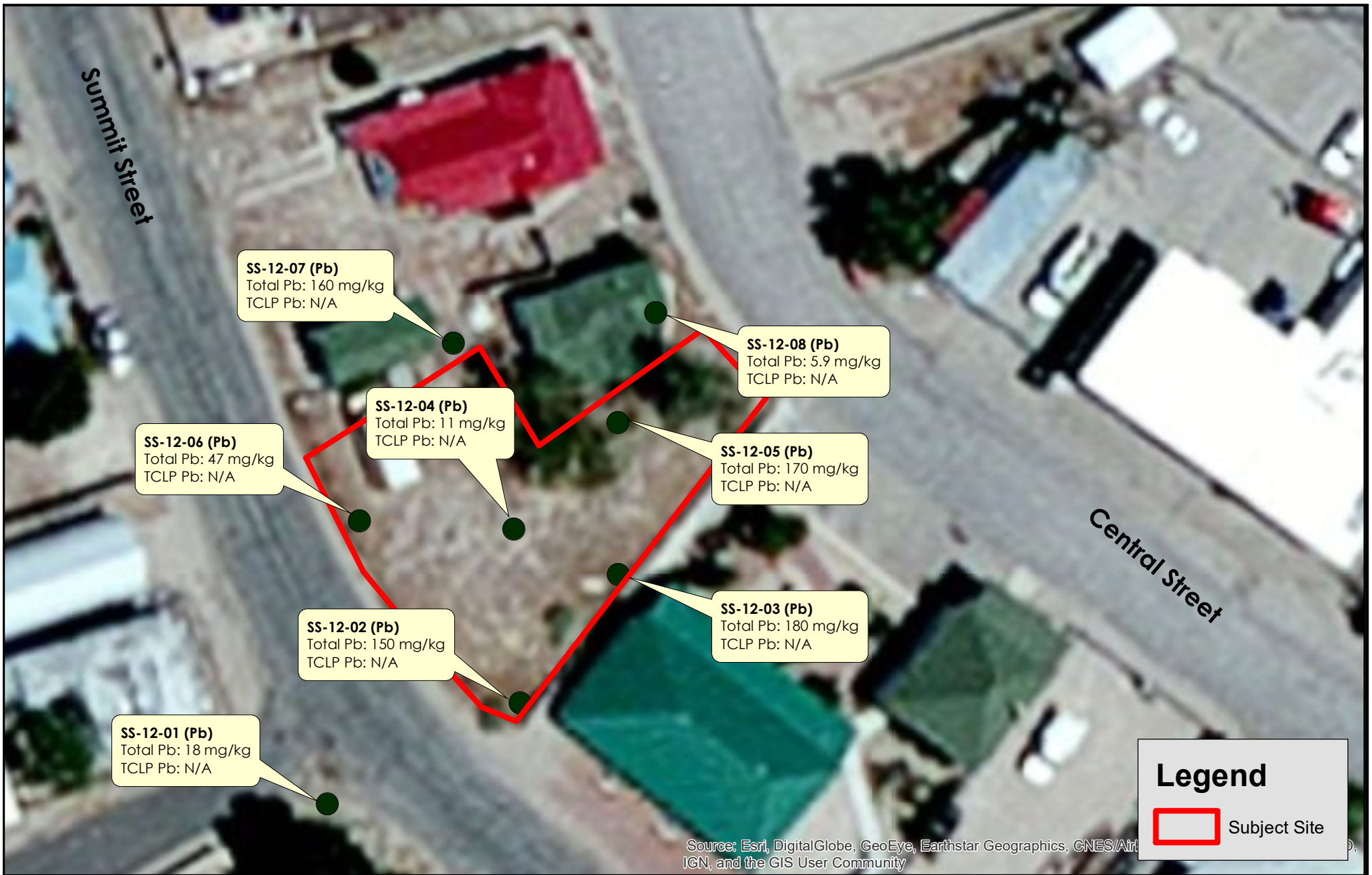
Figure 8 - Pb Soil Samples: 12 inches bgs Tonopah Library Expansion 155 Central Street Tonopah, Nevada
